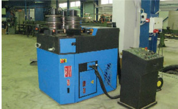
Profile Bending Machine with NC control
