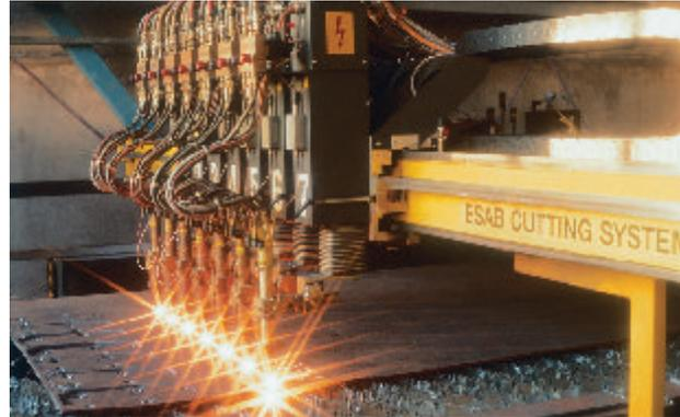
CNC OXY-FUEL Cutting Bench
